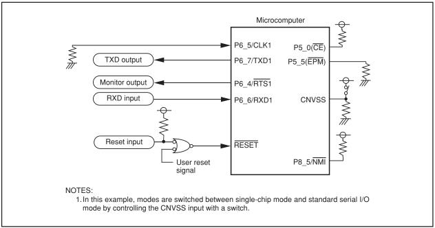
Figure 20.16 Circuit Application in Standard Serial I/O Mode 2
